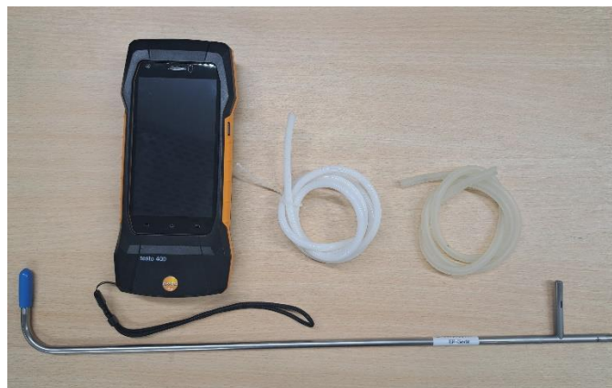
Figure 1: Calibration item: Prandtl pitot tube with measuring instrument (testo 400)
