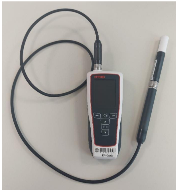
Figure 1: Calibration item: Humidity sensor with measuring device
