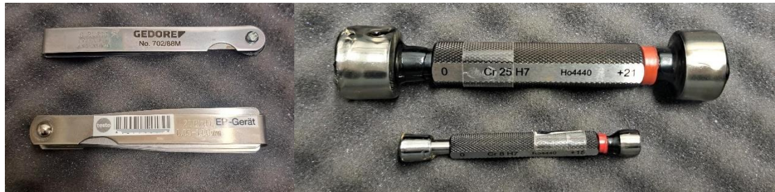
Figure 1: Calibration objects from left to right: 1) feeler gauges, 2) plug gauges
