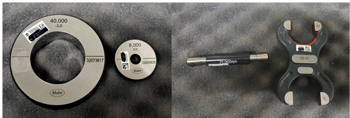
Figure 2: Calibration objects from left to right: 1) setting ring gauges, 2) reference gauge and gap gauge
